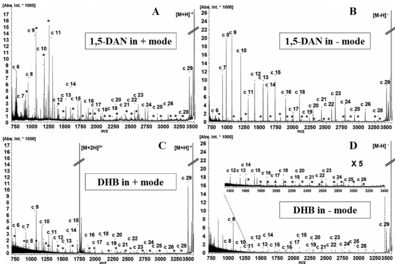
**Figure 2.** reISD spectra of oxidized insulin  $\beta$ -chain (A) in DHB and positive ion mode, (B) in DHB and negative ion mode, (C) in 1,5-DAN and positive ion mode, and (D) in 1,5-DAN and negative ion mode. 1,5-DAN matrix was prepared in  $\text{H}_2\text{O}$  (0.1% TFA)/ACN (1/1). z-Fragments are indicated by an asterisk.
